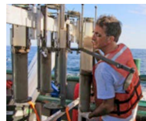
Using a multi-core sediment sampler, David Hastings recovers sediment cores from the Northern Gulf of Mexico. (Photo credit: David Hastings, Eckerd College)
