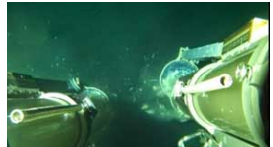
Still shot of the multi-corer as it retrieves sediment cores on the seafloor. Taken during a Deep-C research cruise. Photo credit: Ian MacDonald (FSU).
