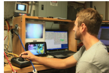
FSU PhD student Chris Malinowski flies the MILET 2-3 m above bottom by reeling cable in or out from the winch.
