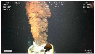
The Macondo well was two days from completion when high-pressure methane gas from the well expanded into the riser, and rose into the drilling rig, where it ignited into an explosion. Experts estimated that oil flowed from the well at a rate of 62,000 barrels per day.
