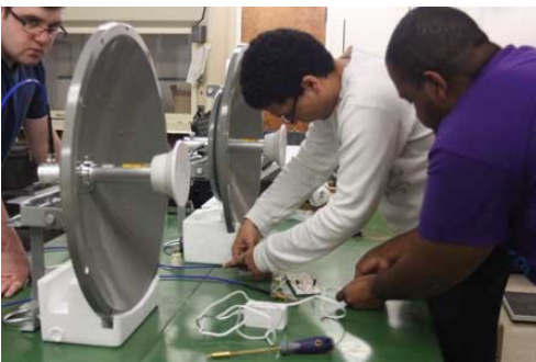
These are the radar antennas that will produce the same signal as the SAR Satellite RADARSAT (5.6 cm, C-Band). (Photo credit: Diana Villa)
