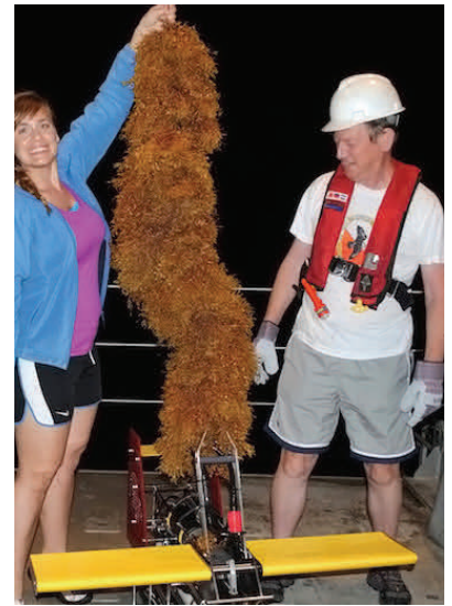
Dr. Piers Chapman (R), Director of GISR, and Ph.D. student Ruth Mullins untangle seaweed from their towed ACROBAT which takes real-time measurements of dissolved oxygen, other chemicals, and physical conditions such as depth, temperature, and salinity. Photo by Steve DiMarco
